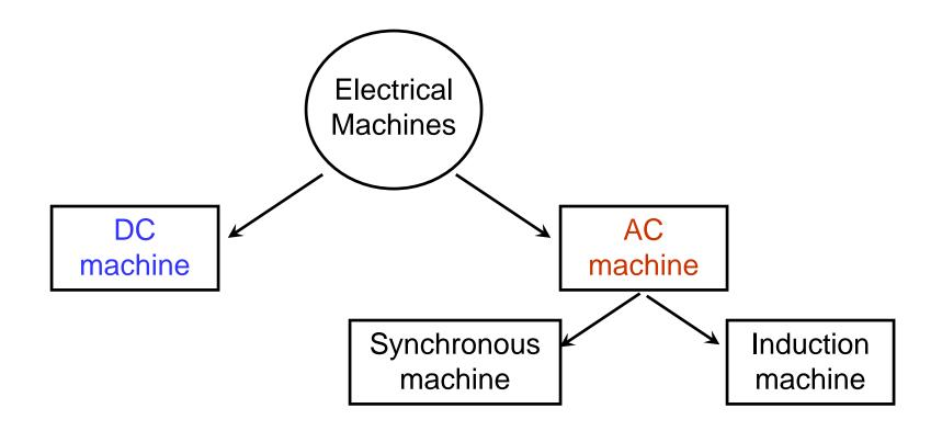
•Machines are called AC machines (generators or motors) if the electrical system is AC.
