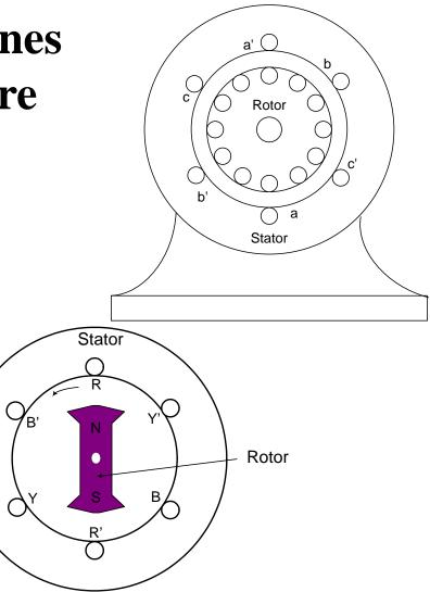
•Both rotor and stator are made of ferromagnetic materials.
